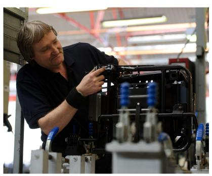
Once the components have been cut the parts are formed, welded and assembled, to make the seat frames. Due to the fast moving and cost sensitive nature of our business, we need to achieve rapid and reliable CNC programming and high levels of material utilization."
