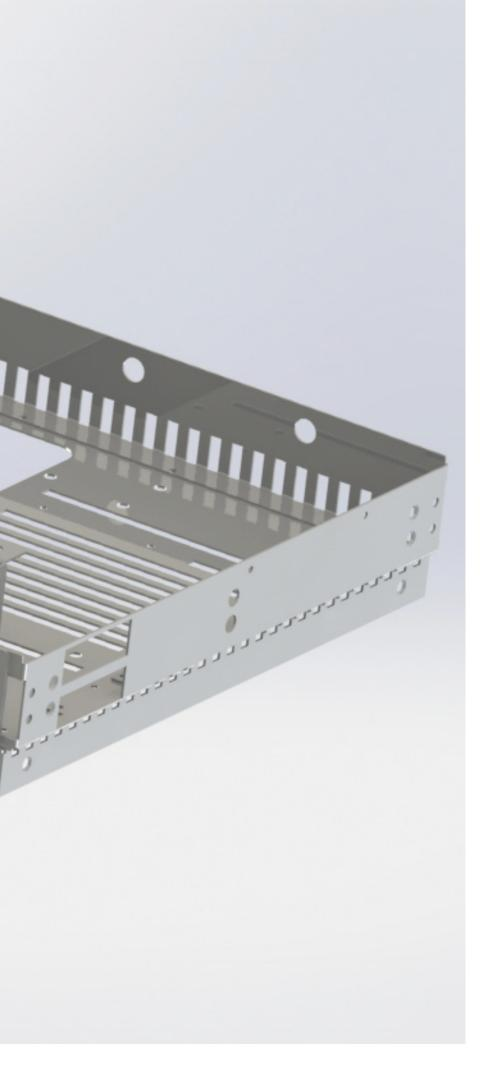
Programming is very fast with Lantek Expert, taking at the most 3-4 minutes to go from the 3D model to the nested CNC programme. Garry Law adds, "The software looks at our library of tools and if there is one available it automatically punches the hole, as this is quicker. Otherwise it generates a laser path. The only decision we have to make is if we want to add microjoints for parts or scrap too big to go down the chute."
